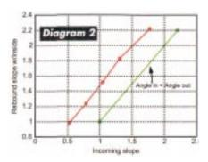
The landing spots were all on the end rail for cue-ball positions from 2 to 6, which went to X and Y respectively. I was surprised to get the cue ball to X for the cut shot shown, but sometimes science does startle. Stated simply, the data say: With pretty good inside follow on a cut down the side cushion, the rebound angle follows "angle in = angle out," provided that you imagine the cue ball starting two diamonds farther up the table.
