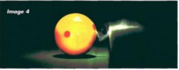
different, though. You can see the hot, bright stick, which points to a hot spot on the cloth. That's where the cue ball was sitting at impact. It jumped on a shallow angle to the next bright spot that looks to be about one or two ball-diameters away, and then there are three or four more shorter jumps as the cue ball settles down on the cloth.
